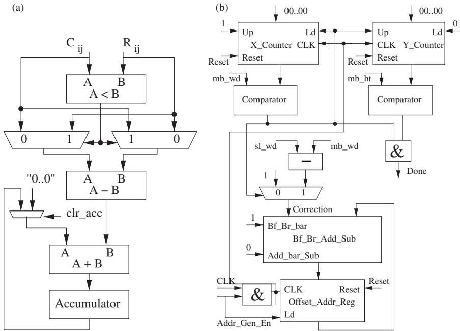
Figure 6. ME using block-matching technique: (a) data-path for SAD computation; (b) hardware schematic representation of AGU for data fetch.
