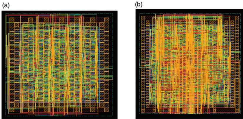
Figure 8. Snapshots of the layouts: (a) 8 bit wide CAGU; (b) 8 bit wide DRDP.
