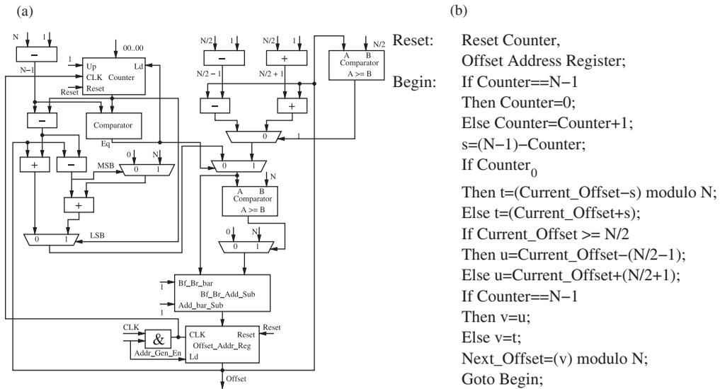
Figure 5. (a) Hardware schematic representation and (b) algorithm for data fetch AGU for linear-phase FIR filter kernel AGU – streaming data.
