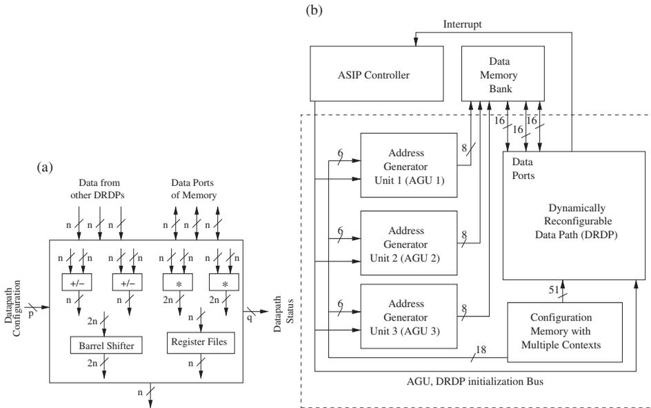
Figure 1. Block schematic diagram of reconfigurable functional unit with its components: (a) proposed dynamically reconfigurable datapath unit (RDPU); (b) reconfigurable functional unit.
