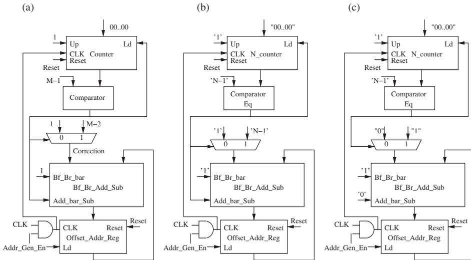
Figure 3. Hardware schematic representation of AGU used by convolution kernel: (a) Data fetch – stored data, (b) coefficient fetch, (c) storage of result.
