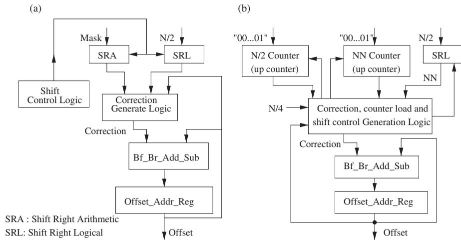
Figure 2. Hardware Schematic of AGUs used by FFT kernel: (a) Hardware schematic representation of bit-reversed address generator; (b) Hardware schematic representation of FFT twiddle-factor address generator.
