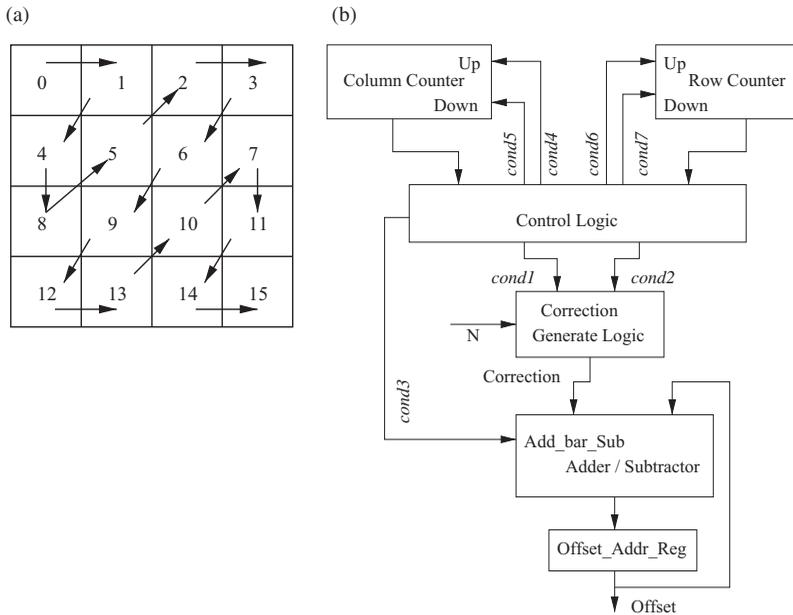
Figure 7. (a) Sequence of addresses and (b) hardware schematic representation of AGU for zig-zag addressing mode.
