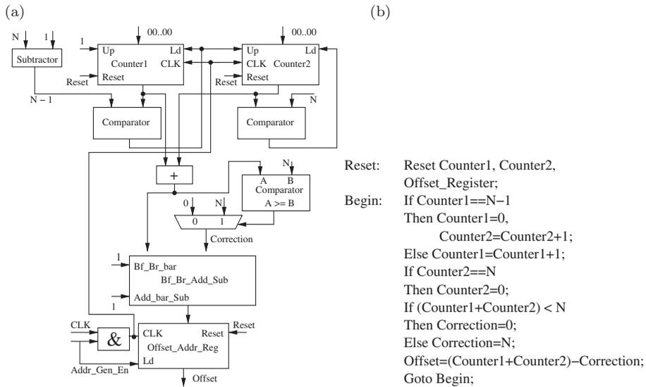
Figure 4. (a) Hardware schematic representation and (b) algorithm for data fetch AGU for convolution kernel – streaming data.
