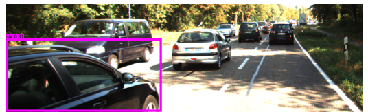
Fig. 9. Output from the hardware implementation of 13 \times 13 arm of TinyYOLO-v3 architecture, as obtained in RTL simulation
