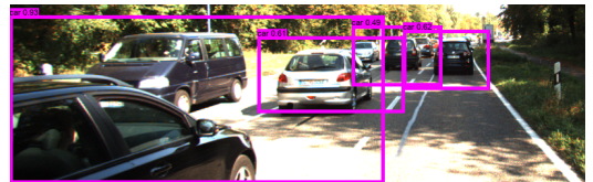
Fig. 8. Output from the hardware implementation of 26 \times 26 arm of TinyYOLO-v3 architecture, as obtained in RTL simulation
