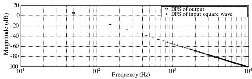
**Figure 11.** Frequency spectrum of the input and output depicting the total absence of harmonics (O) in the output and exact matching of amplitudes of the input (+) with that of the output (O) at the fundamental frequency (50 Hz).
