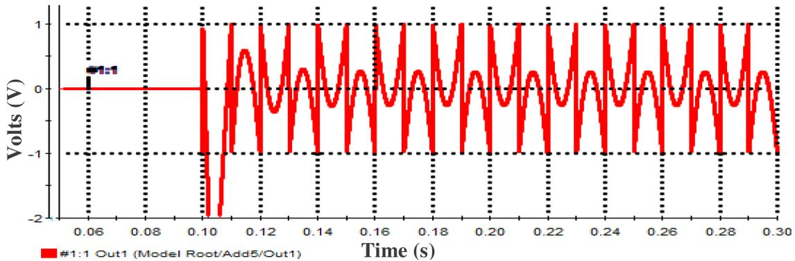
Figure 10. Harmonics extracted from a square-wave input.
