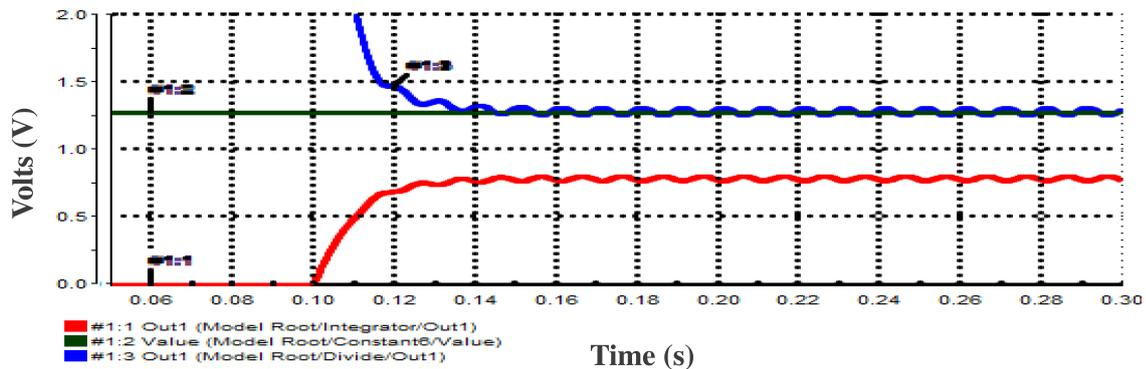
Figure 8. Step response showing settling time for a square-wave input:  $1:1 \leftrightarrow u$ ,  $1:2 \leftrightarrow \frac{4}{\pi}$ ,  $1:3 \leftrightarrow c$ .
