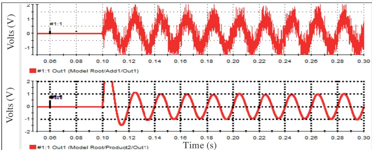
**Figure 13.** Performance under noisy conditions: top – noisy input; bottom – filtered output.
