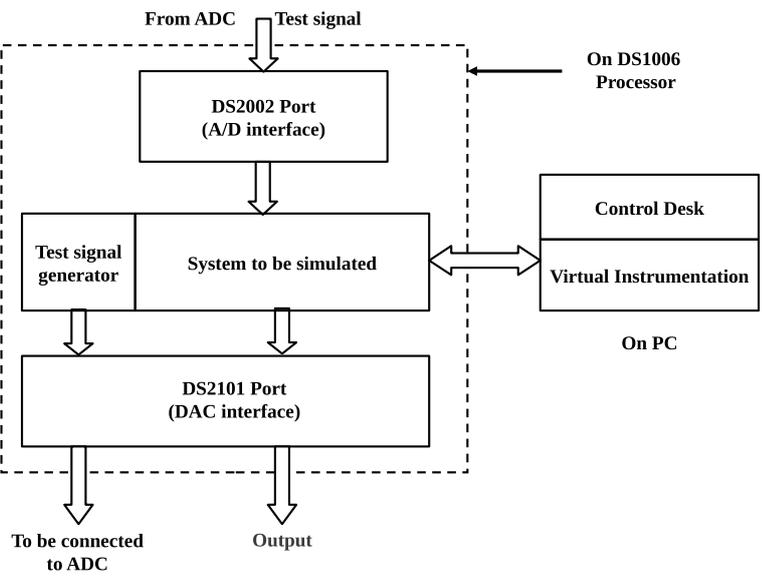
Figure 6. Real-time experimental setup schematic.
