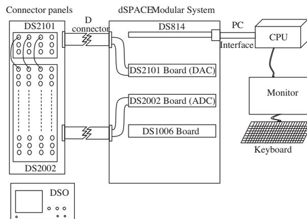
**Figure 3.** Schematic of DS1006-based modular system.
