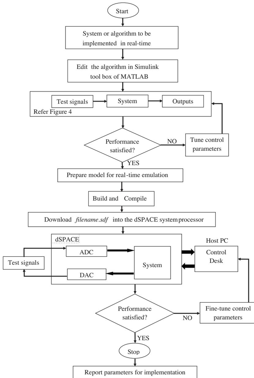
Figure 5. Schematic for the process of validating the algorithm on a real-time hardware-emulation platform.
