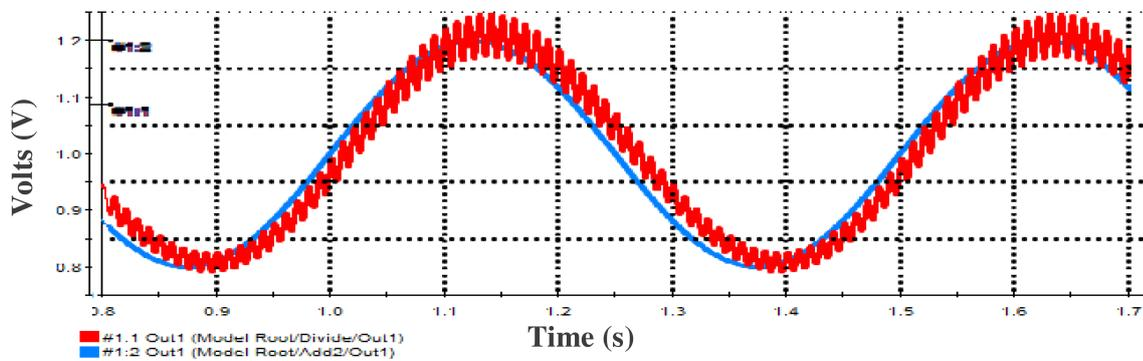
**Figure 12.** Output amplitude to an input whose amplitude is modulated: blue – input; red – output.
